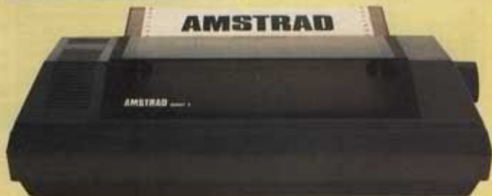
Optional 80 column dot matrix printer DMP-1 operates at up to 50 characters per second. Combined with the CPC464, it offers a high performance text processing system for only £199.95.
